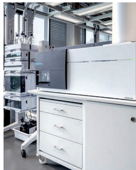
A LC-ESI-Q-TOF mass spectrometer (6545XT, Agilent) has been installed in October 2023 at the IBS mass spectrometry platform.
